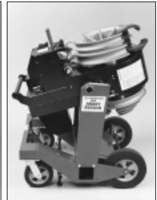
Balanced bending head pivots easily as it is changed from the vertical bending position to the horizontal bending table position.
