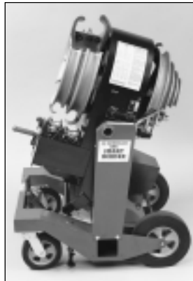
Balanced bending head pivots easily as it is changed from the vertical bending position to the horizontal bending table position.
